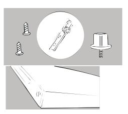
4) Remove the plastic cover from door hinge first. Then unscrew the two screws from top bracket and replace on the other side.
